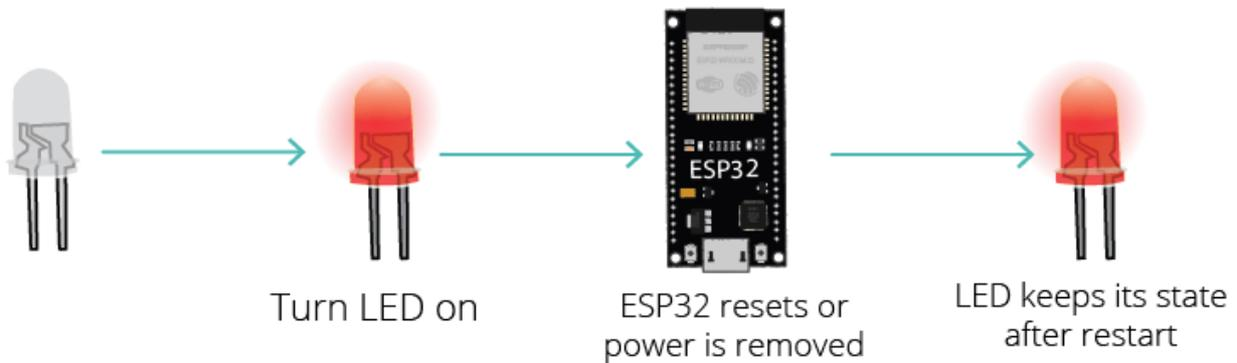
We'll show you an example using an LED and a pushbutton. The pushbutton controls the LED state. The LED keeps its state between resets. This means that if the LED is lit when you remove power, it will be lit when it gets powered again.
