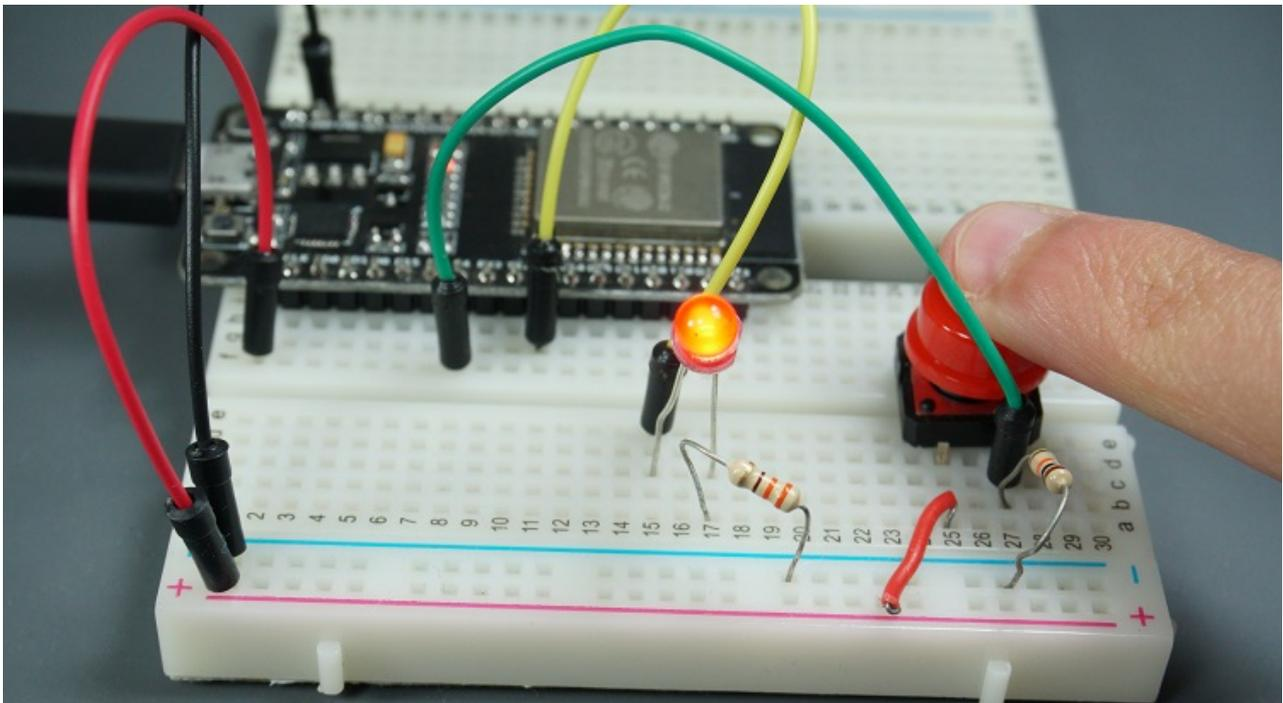
When the ESP32 restarts, it will read the last state saved on Preferences and set the LED to that state. It also prints a message on the Serial Monitor whenever there's a change on the GPIO state.
